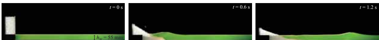
Figure 1: Three successive images separated by the same time interval \Delta t = 0.6 s from the time origin t = 0 (left image) where the granular column (aspect ratio a = 2.5 and mass M = 3.9 kg) of d = 5 mm glass beads is released by the gate opening and fall into water of depth h_0 = 55 mm.
